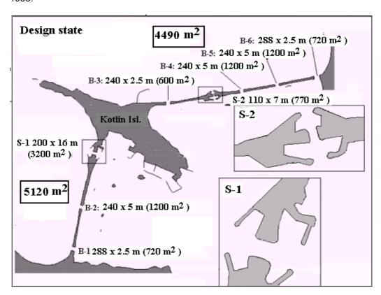
Figure 3: Design of the St. Petersburg Flood Protection Barrier (approved western variant)
