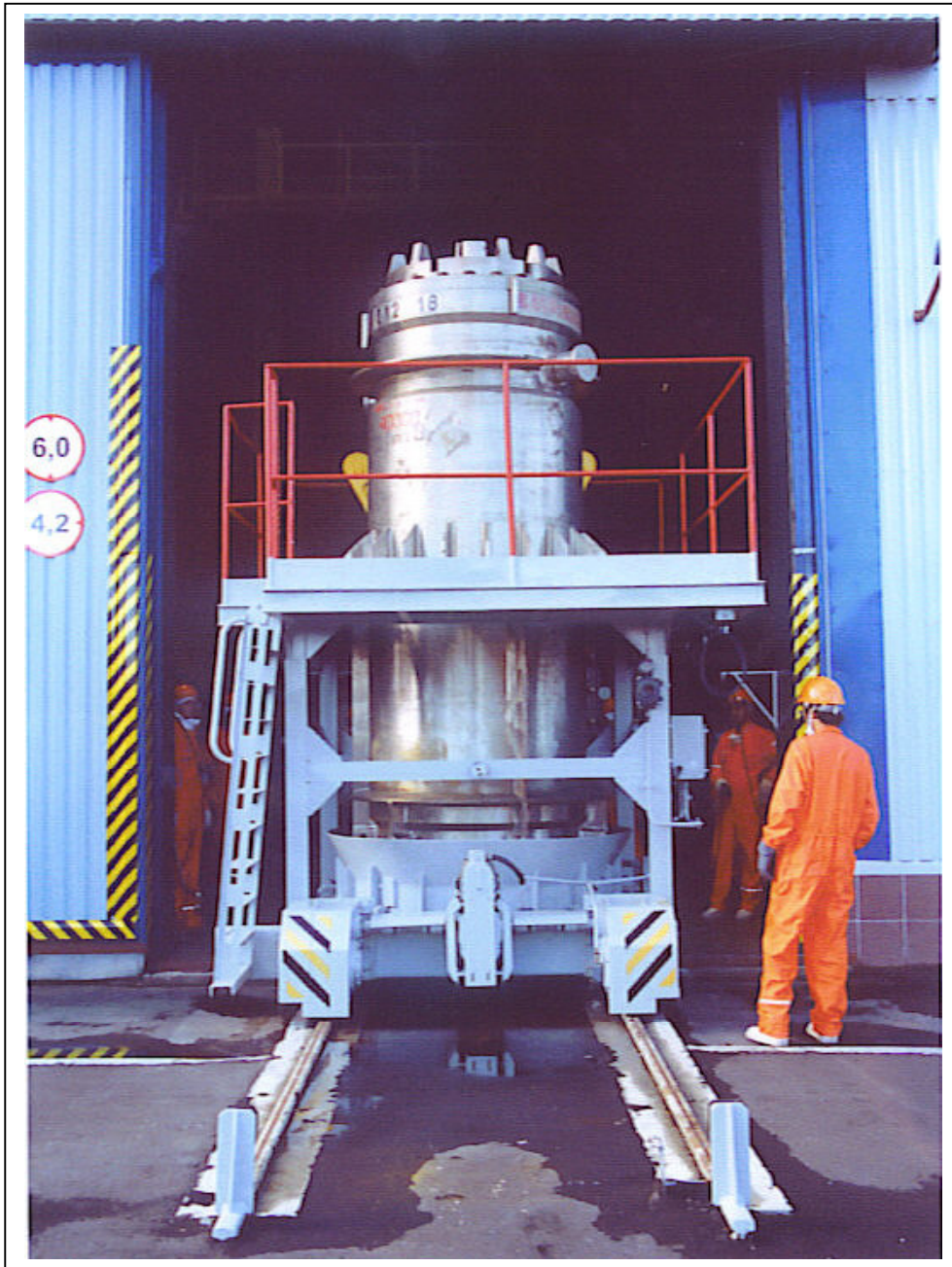
Figure 2.1.4-2. Spent Nuclear Fuel Storage Pad at Zvezdochka shipyard. Transfer of TK-108 fuel cask.
