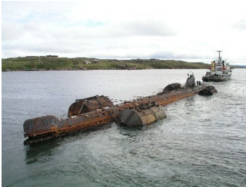
Figure 4.2.1-1 Towing of K-159 with Floatation Assistance
