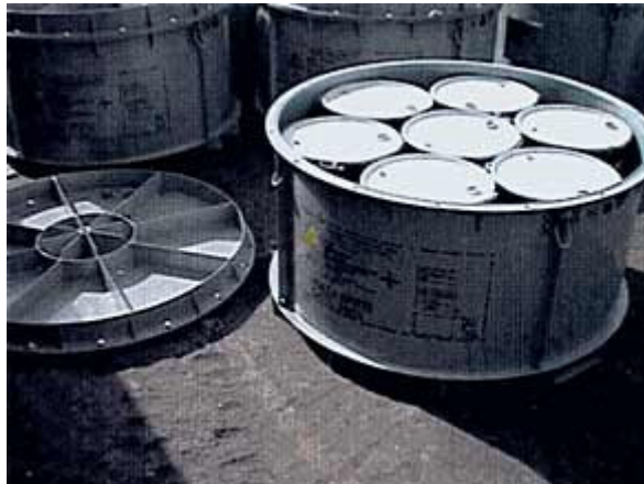
Figure 2.1.4-4: AMEC Radioactive Waste Storage and Transport Container
