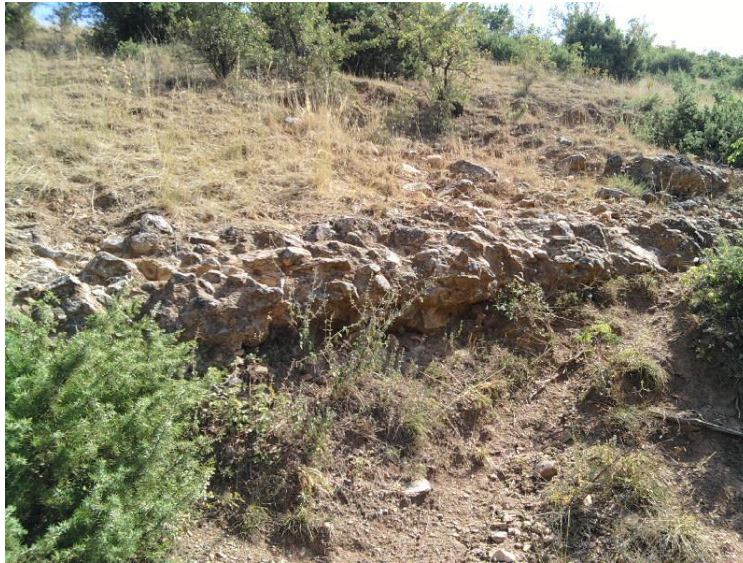
Picture 12 Limestone breccia before the village Kamen Dol (start of new designed bridge)
