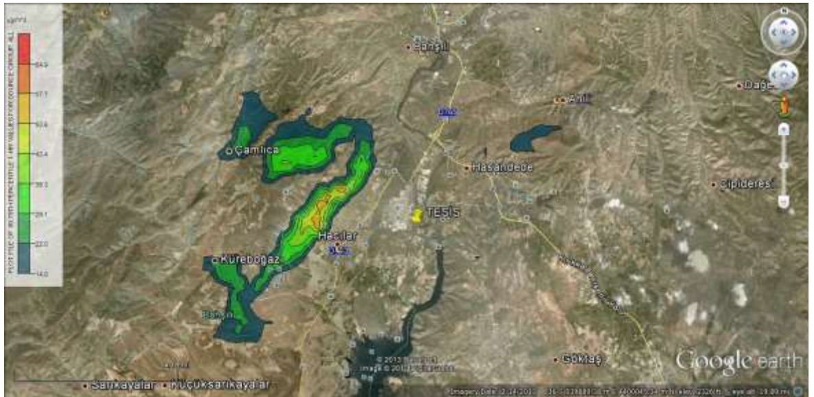
Figure 10. Hourly Average GLC Dispersion of NO 2 for TPP
