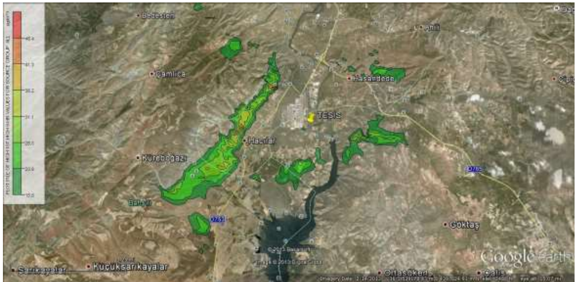
Figure 23. Daily 8 Hours Average Maximum GLC Dispersion of CO for Cumulative Scenario (Scenario-4)
