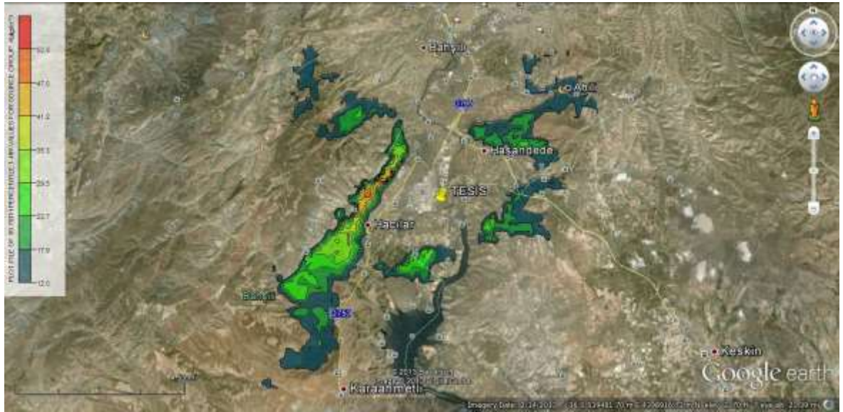
Figure 4. Hourly Average GLC Dispersion of \text{NO}_2 for KCPP (Scenario-1)
