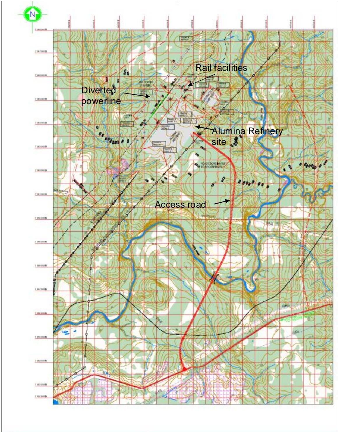
Figure 3: Plan of proposed refinery site "early works" (not to scale)
