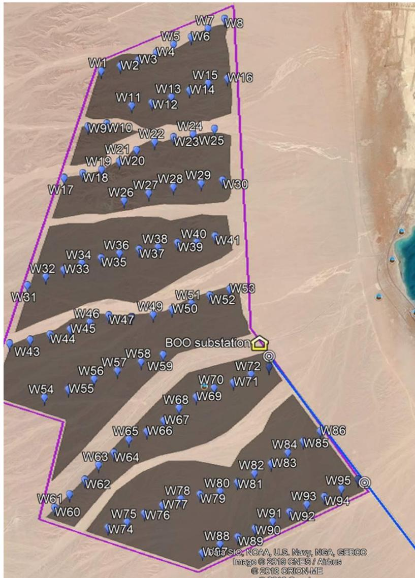
Figure (1): Configuration based on 96 turbines rated 2.6 MW
