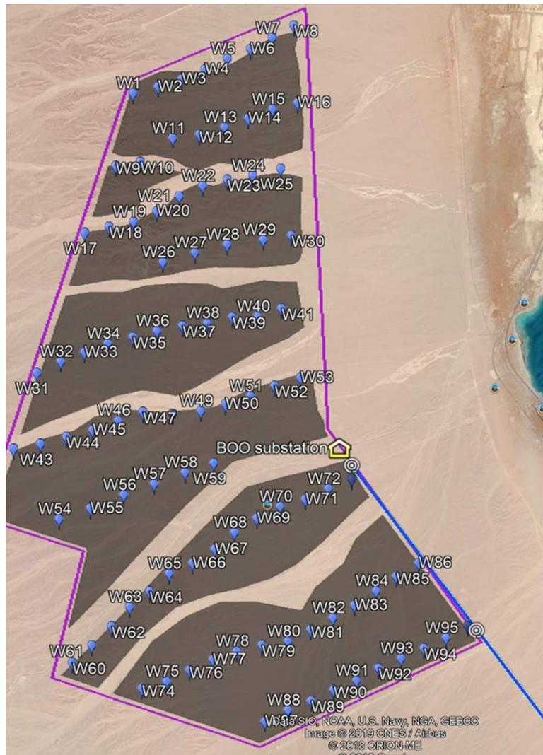
**Figure (5): Lekela project layout (96 x 2.6MW)**
