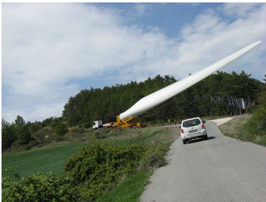
Slika 9: Transport kraka vetroturbine planinskim putem
