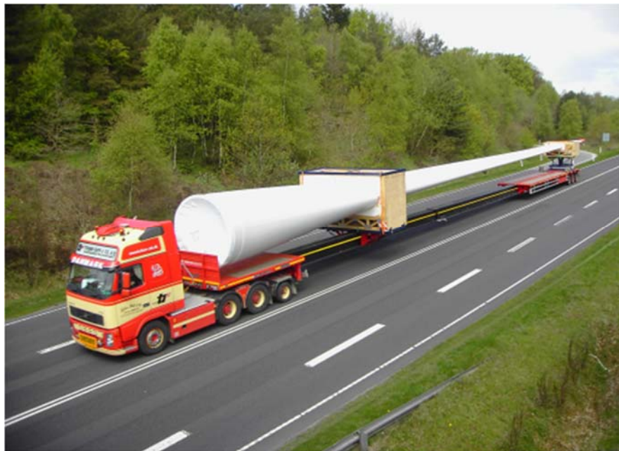
Slika 8: Transport kraka vetroturbine autoputem
