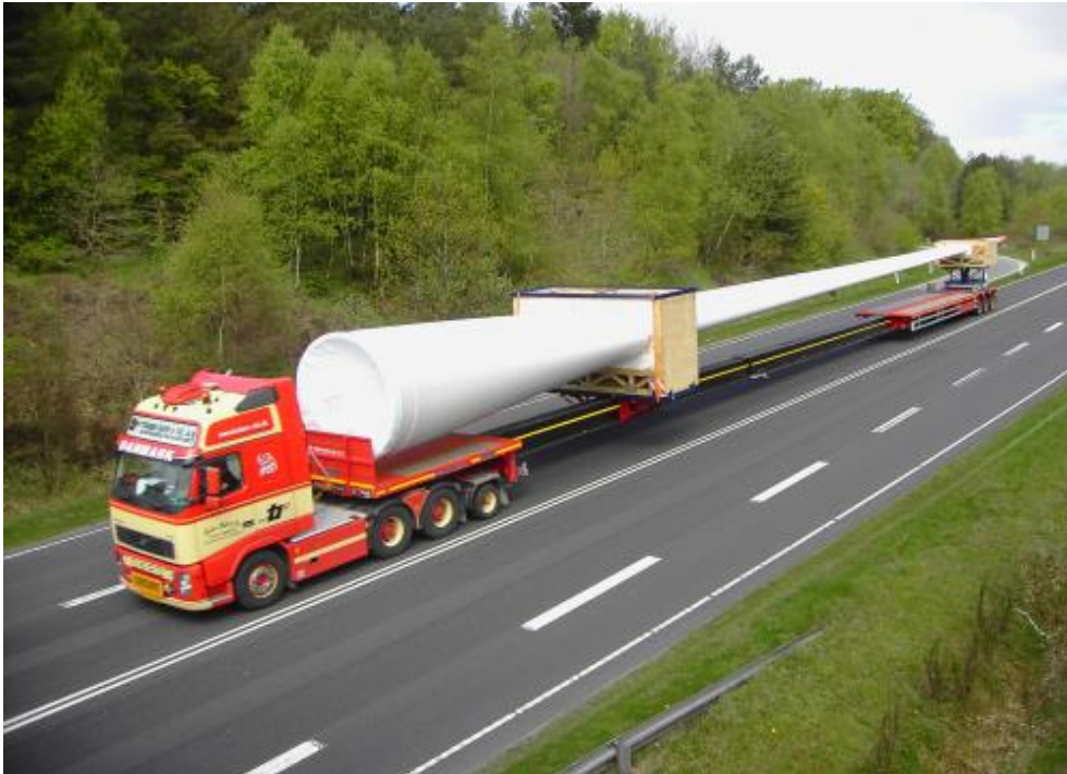
Figure 8: Blade transport on highway
