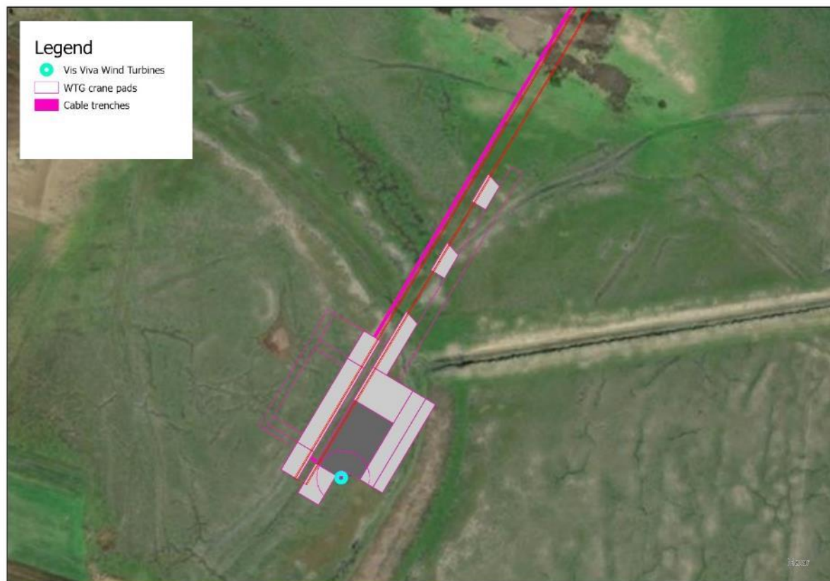
Figure 2-4 Typical WTG and Associated Working Platforms
