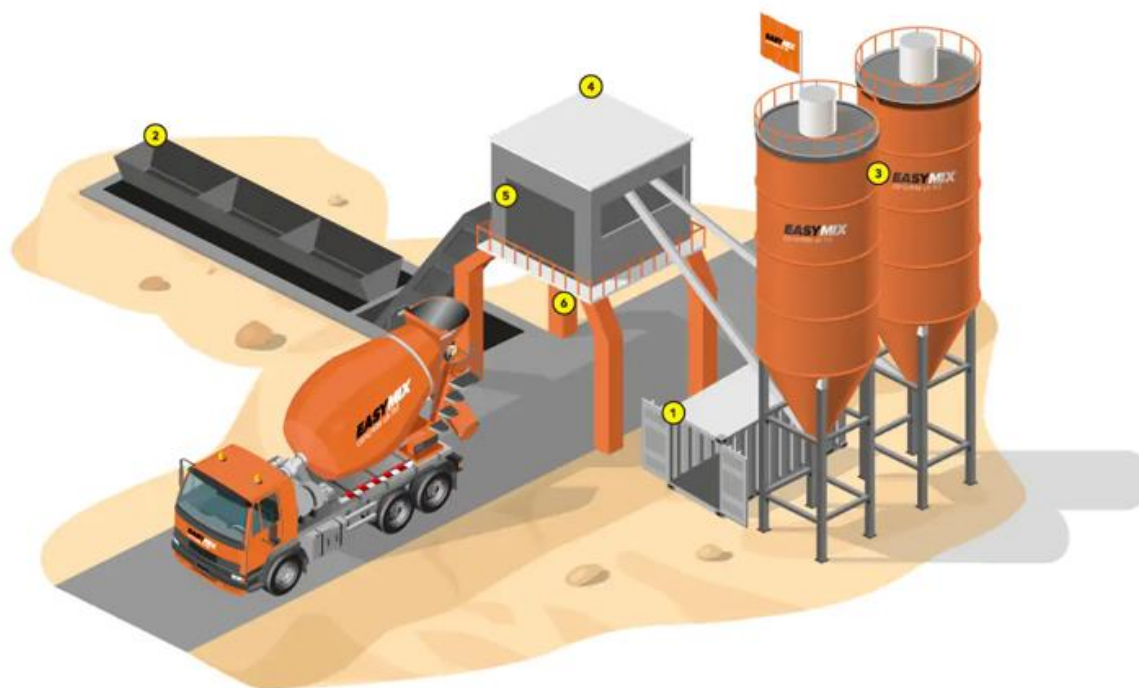
Figure 2-6 General Concrete Batching Station Operation Scheme
