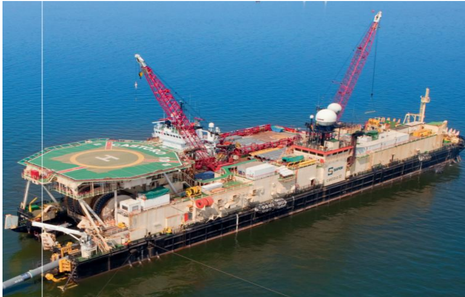
Figure 6-42: Typical Pipelay Vessel (S-Lay Method)
