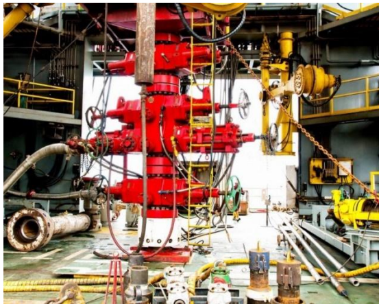
Figure 6-52: Typical BOP Mechanism on a Jack-Up Rig
