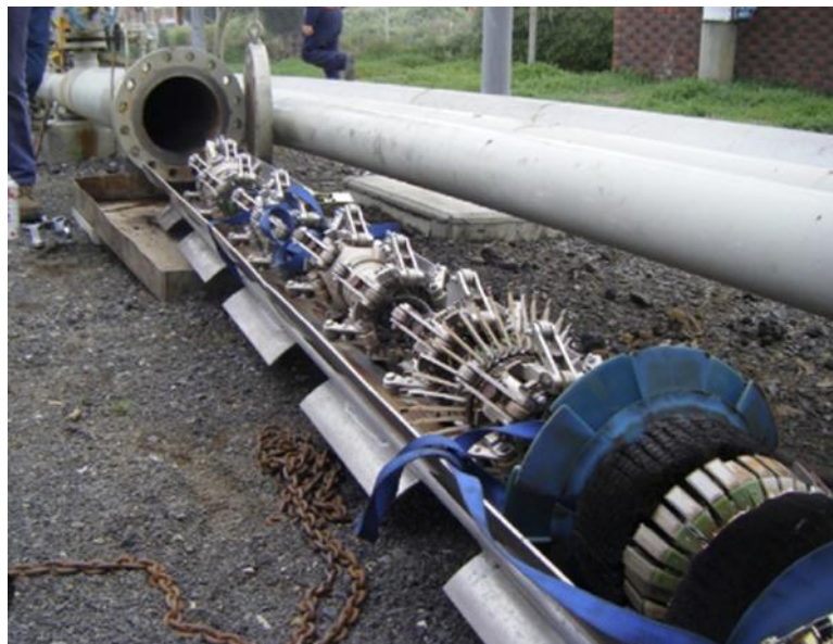
Figure 6-45: Pipeline inspection equipment (Intelligent pig)
