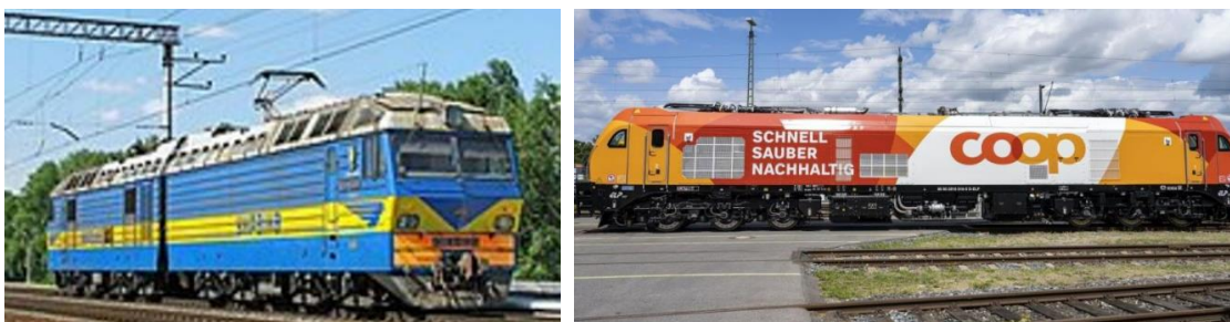
Picture A.2.2 Two-Section Electric Locomotive vs. Single Section Model
