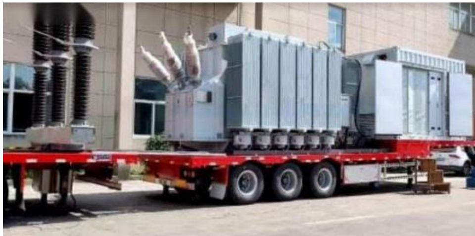
Figure 140: Example of vehicle delivering transformer
