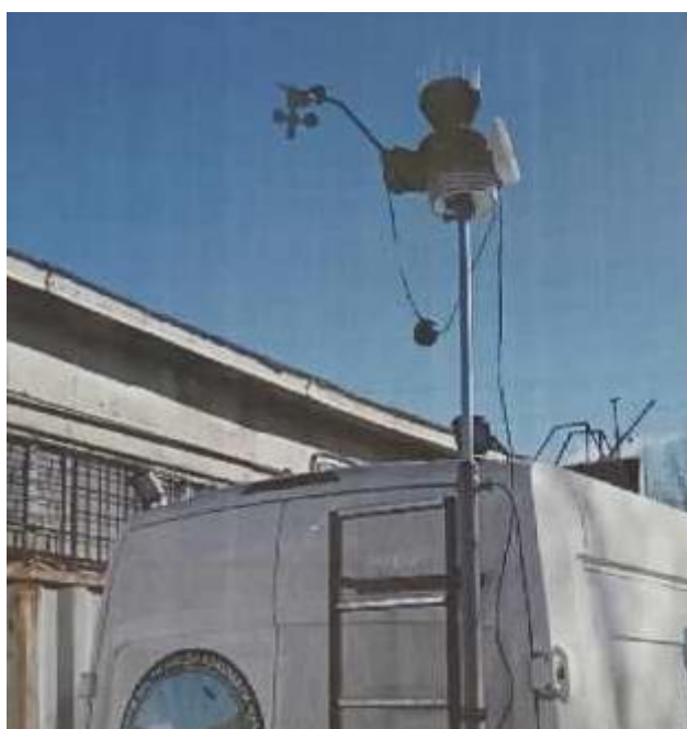
Photo 4. Installation for measuring climatic conditions of the region (wind speed, air pressure, humidity, wind direction, temperature)
