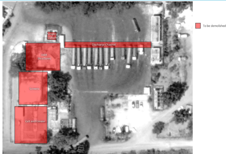
Figure 9: Components to be Demolished for Decommissioning of the Tanker Discharge Station
