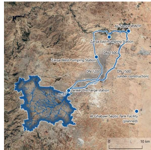
Figure 6: Overview of Wastewater Treatment and Conveyance Facilities
