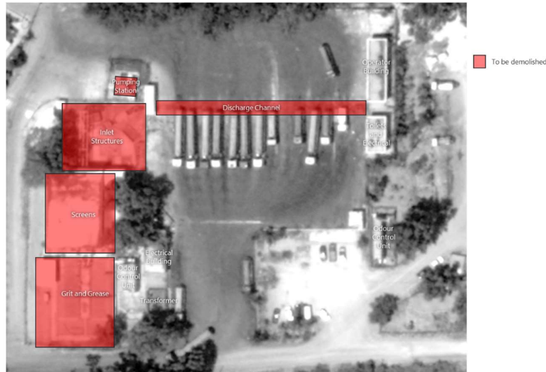
Figure 10: Components to be Demolished for Decommissioning of the Tanker Discharge Station
