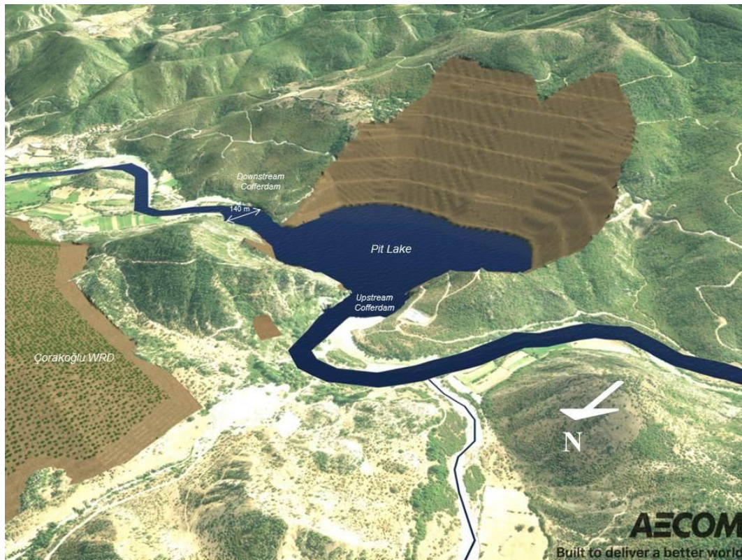
Figure 5-4 Conceptual closure scenario for the open pit to be flooded by the Gökırmak River
