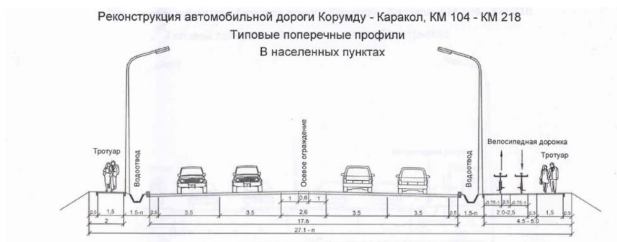
Figure 2-5. Cross-section with separate bike path
