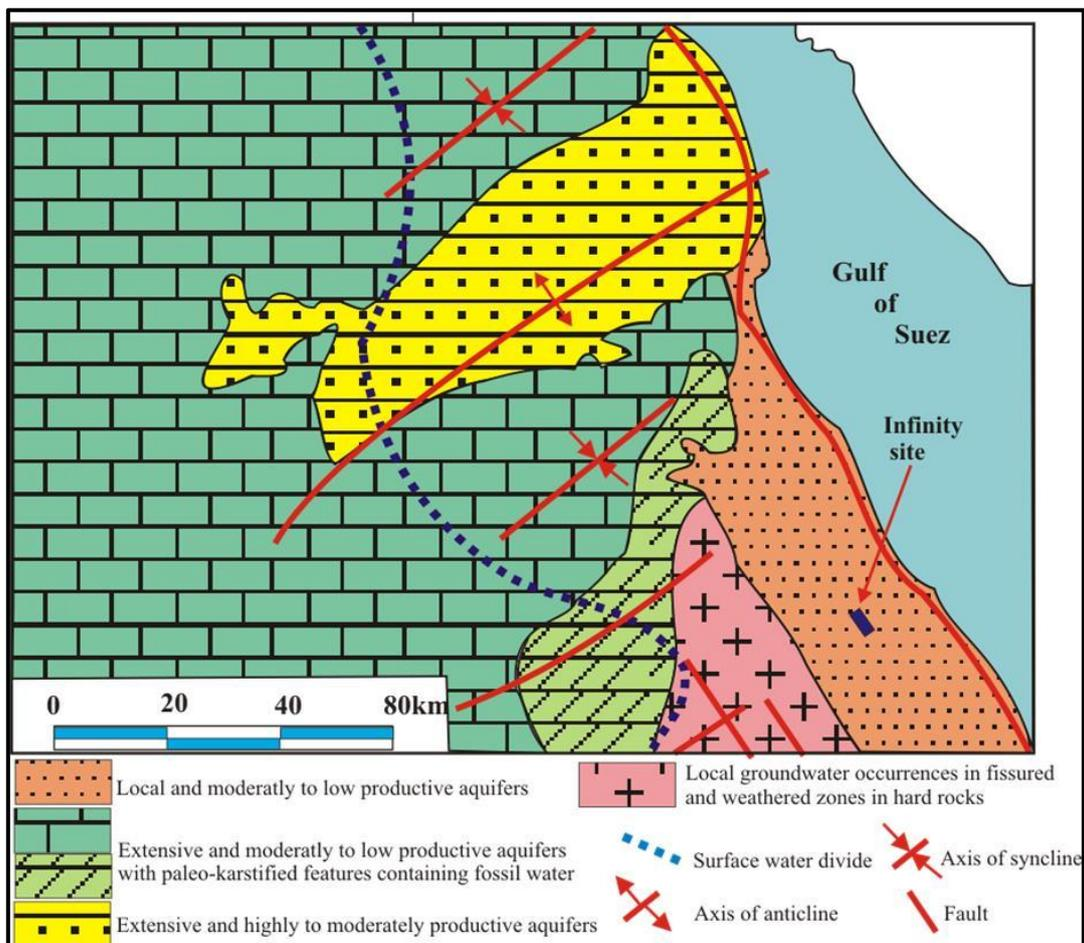
Figure 24: Hydrogeological Map of the Area around the Project Site
