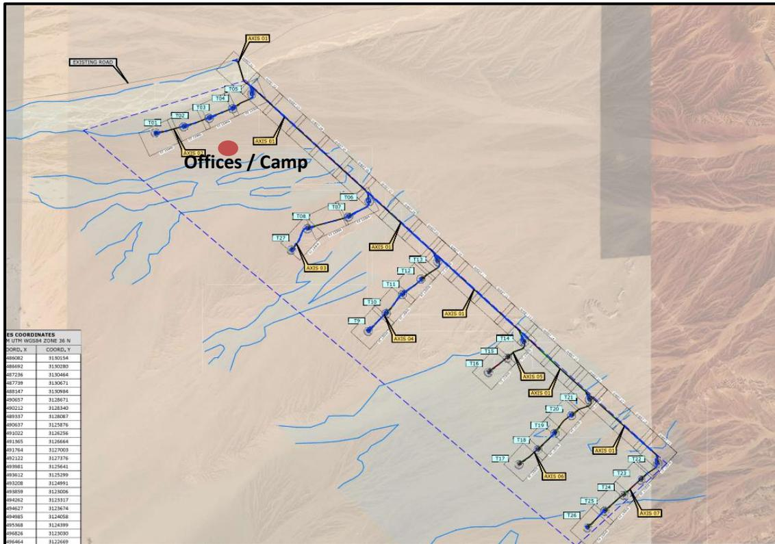
Figure 11: Camp, Offices and Access and Internal Road Network
