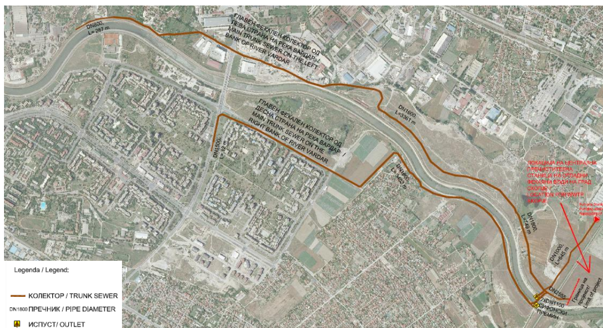
Picture 13. Map of Trunk Sewer on Left and Right Bank of the Vardar River, Siphon and WWTP Location (source: Book 2 Detailed Design of Siphon Crossing below the Vardar River and Connection to the WWTP)
