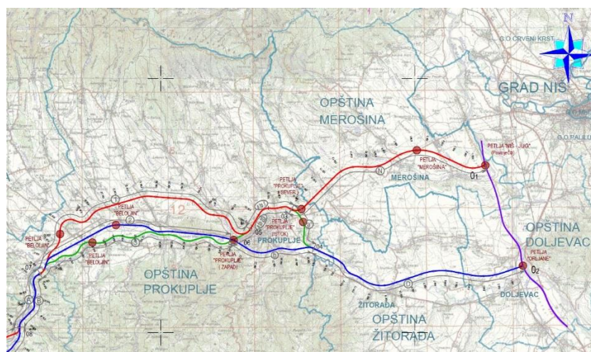
Figure 8 Variants of the highway route processed in the General Design
