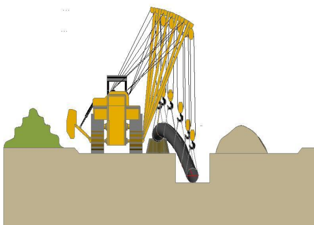
Fig. 1.X. Schematic view of gas transmission pipeline laying (left) and view from the construction site (right)
