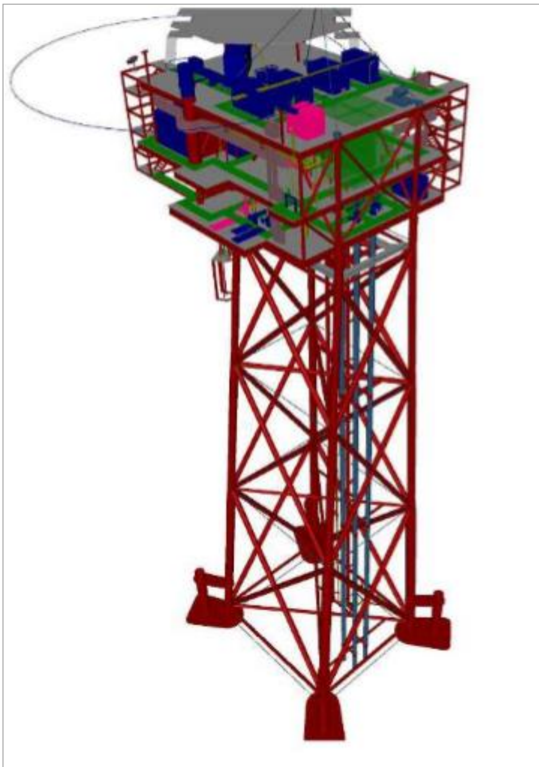
Figure 5.2 Ana platform schematic. The platform is oriented with “platform North” being rotated 30° clockwise from true North as shown in Figure 5.3.
