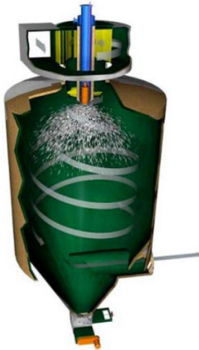
Figure 15. Reactor for semi-dry desulfurization by Keppel Seghers
