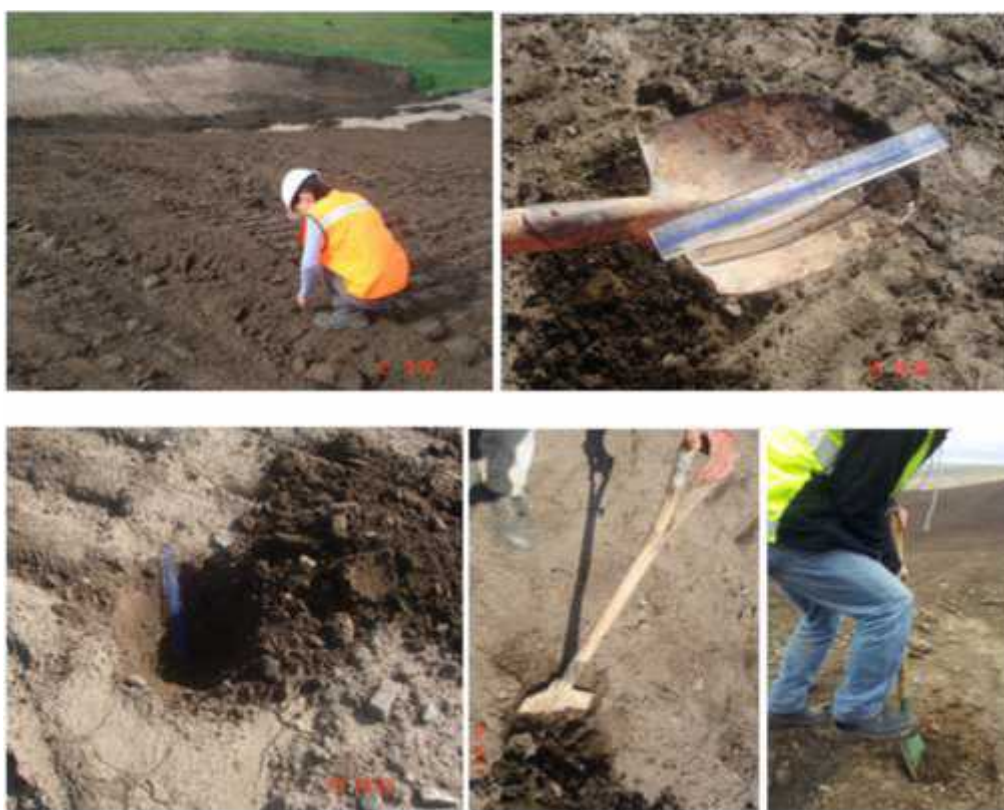
Image 5.7. Measuring thickness of topsoil layer
