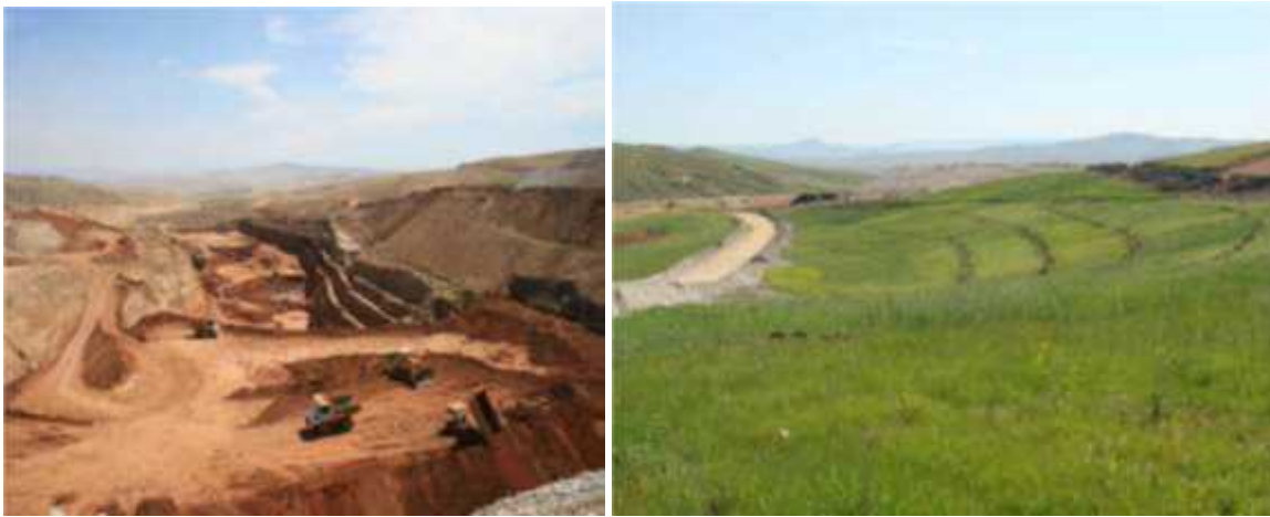
Image 5.3. Placer deposit extraction before and after reclamation
