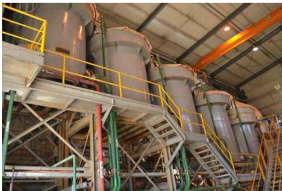
Image 3.12. CI carbon absorption unit
