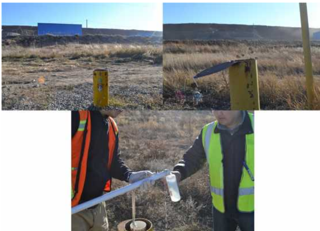
Image.6.2. Monitoring wells near heap leach pad and sampling process
