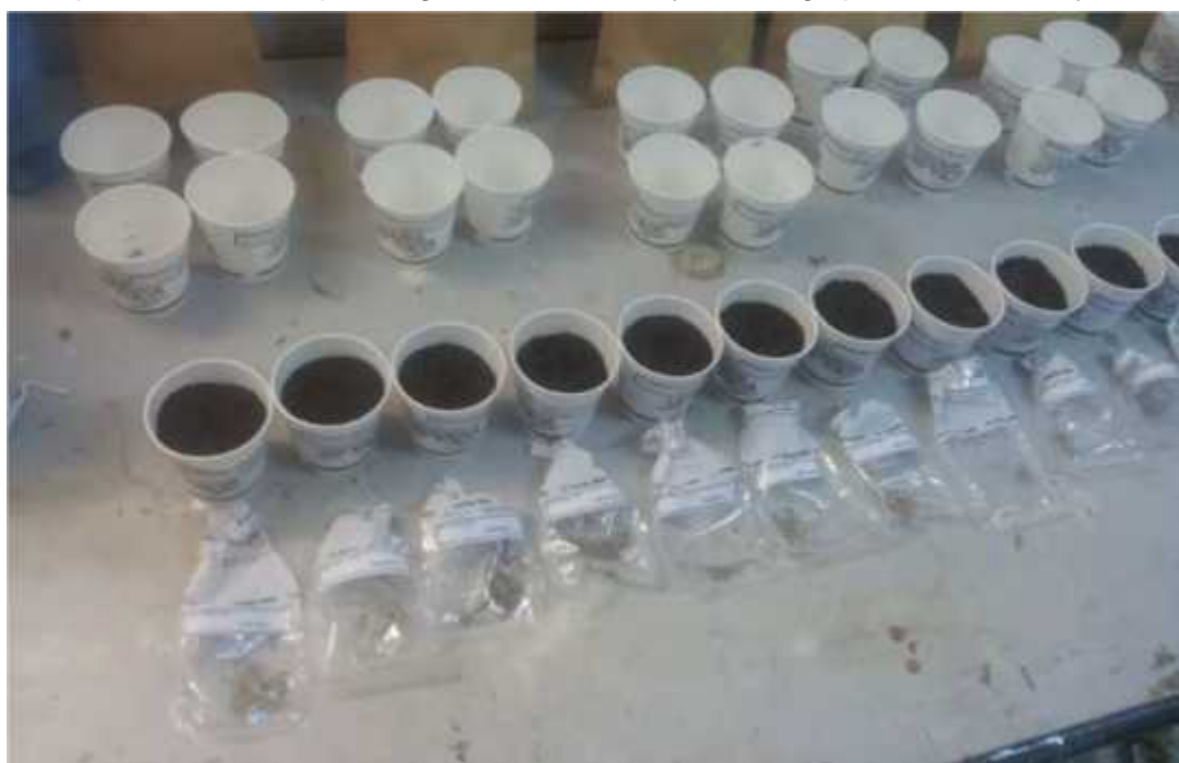
Image 5.10. Seeds prepared for indoor test to defined sprouting rate
