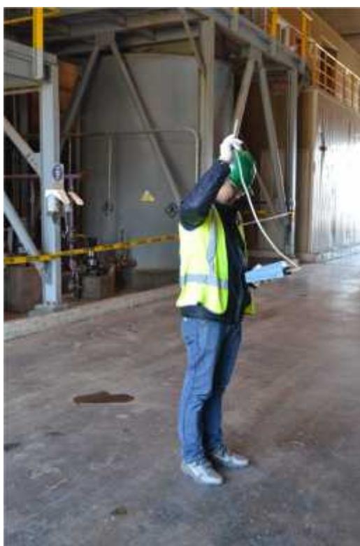
Image 4.5. Dust measurement in the mill using dust measuring DUSTTRACK device
