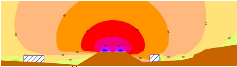
Figure 6.3.9-01: Road on an embankment without noise protection measures – cross-sectional view with isophones (noise contour plots)
