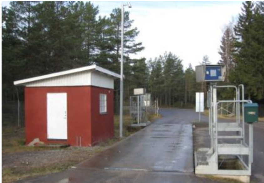
Figure 29 Illustration of a weigh-bridge including a registration system (note the camera on the top of the pole)
