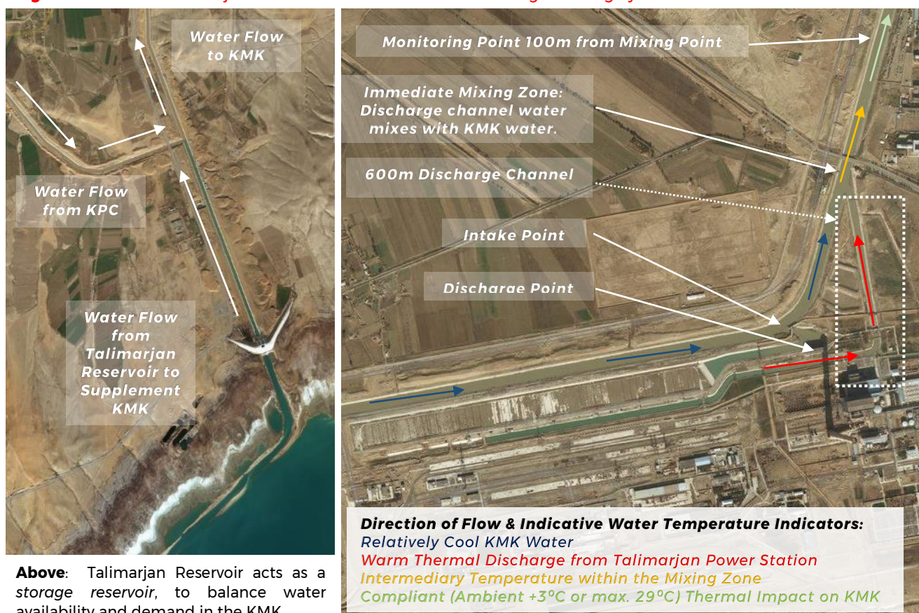
Figure 4: KMK and Talimarjan Thermal Power Station Once-through Cooling System
