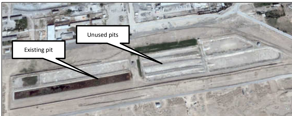
Figure B-6: Aerial Image of Existing Sludge Pits
