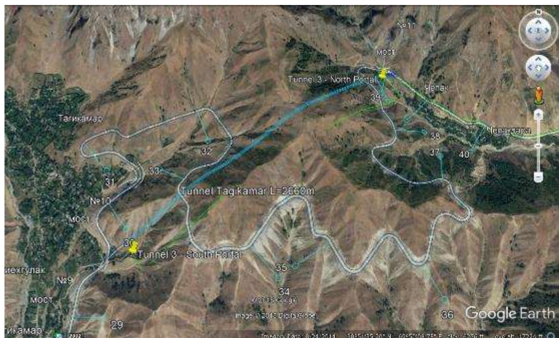
Figure 17: New Third Tunnel (Tagikamar) – showing earlier “high pass” no tunnel option
