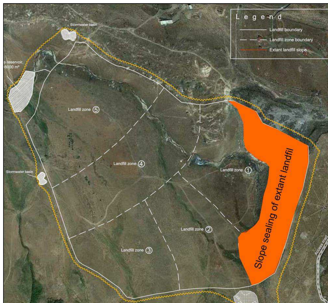
Figure 3: Affected area of slope sealing for extant landfill of new landfill zone 1 and new landfill zone 2 (source: Technical Feasibility Study, 2012)
