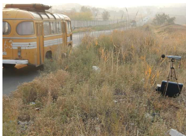
Figure 10: Noise measurement, 4 m from the road axis
