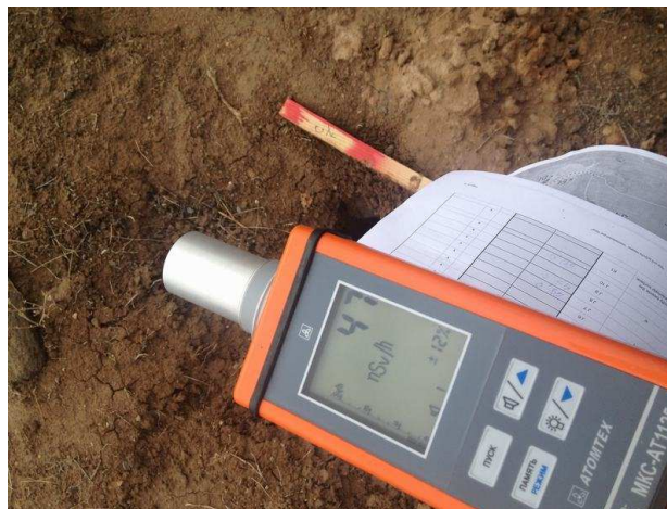
Figure 52: Measurement of radioactivity at point J7 (this is the location of borehole BH 7)
