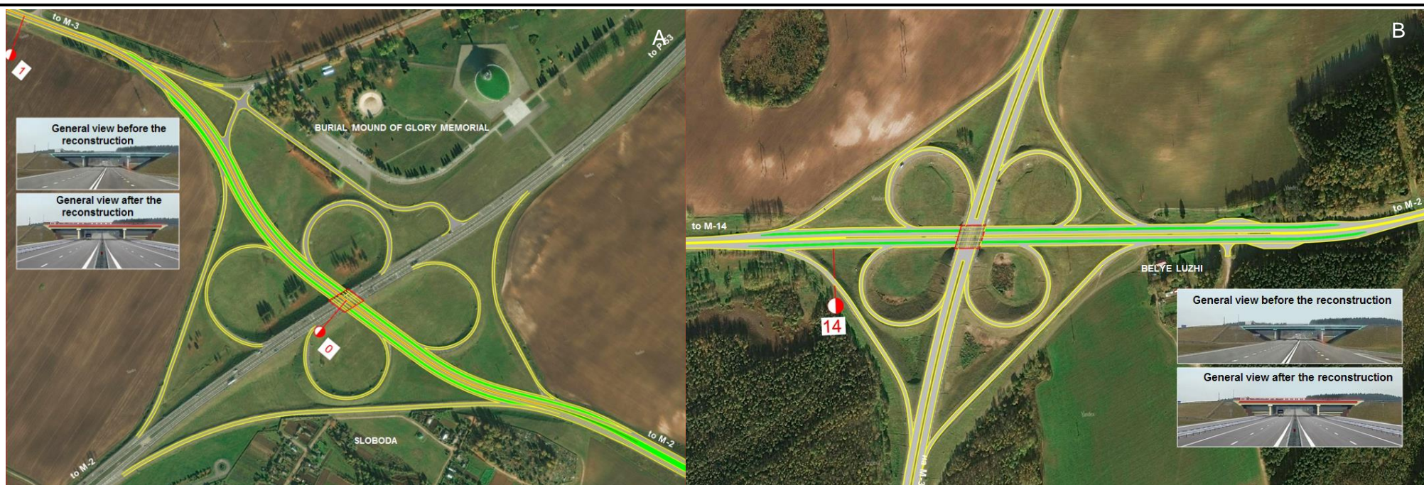
Figure 2.2-2 Schematics of intersections reconstruction (A) at M-2 motor road crossing and (B) at M-3 motor road crossing
