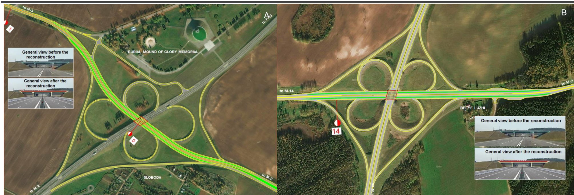
Figure 2.3-2 Schematics of intersections reconstruction (A) at M-2 motor road crossing and (B) at M-3 motor road crossing
