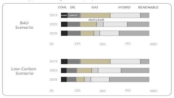
Chart 22: Turkey power: installed generation capacity under BAU and low-carbon scenarios
