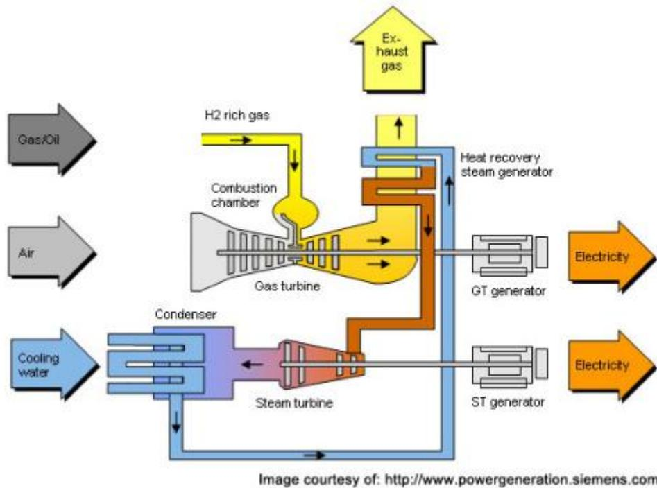
Figure 2-1 Diagram of the CCGT process
