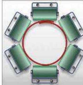
Figure 3 – Pipe conveyor section
